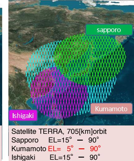
Combination of the three antenna coverage area are similar to Single big antenna one.
